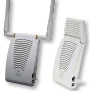
supports external antennas through dual, detachable antenna interfaces and the AP-61 supports dual, integral, high-performance omni-directional multi-band antennas.
