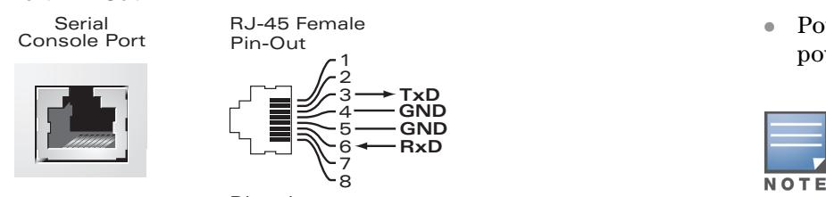
**Figure 8** RJ-45 (Female) to DB-9 (Male) Modular Adapter Conversion
